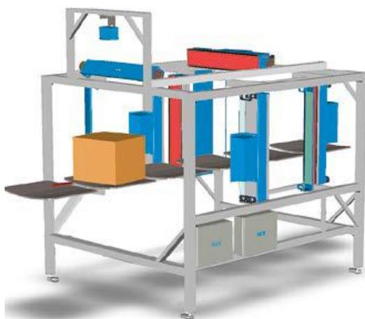
Fig. 8. 5-way scanning with 5 cameras<sup>13</sup>
