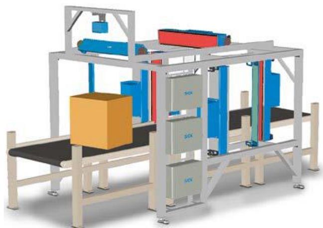
Fig. 9. Scanning which combines volume measurement, weighing and recognition<sup>14</sup>
