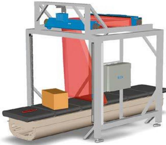
Fig. 6. Positioning the camera above the object to be identified<sup>11</sup>
