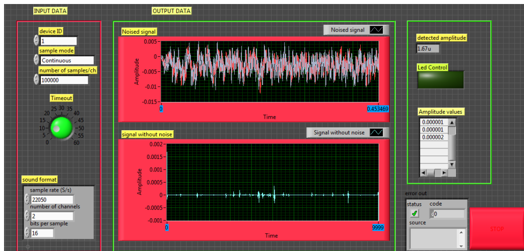
Fig. 5. System acoustic response using wavelet denoising method (there is no force applied to the system)
