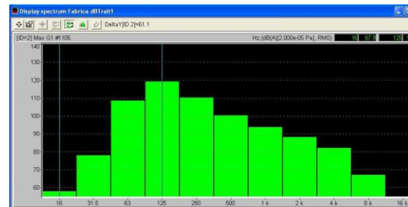
Fig. 5 Noise evaluation in the middle of the parking lot on Invatatorilor Alley (“M. Eminescu” school) between 7:45 and 8:00 AM (22 Oct 2012)
