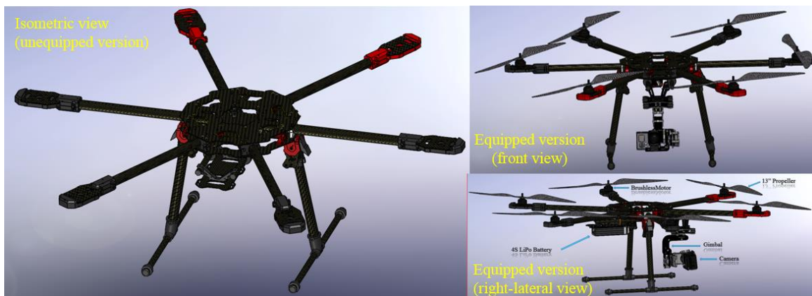
Fig.8 The CAD prototype of the hexacopter
